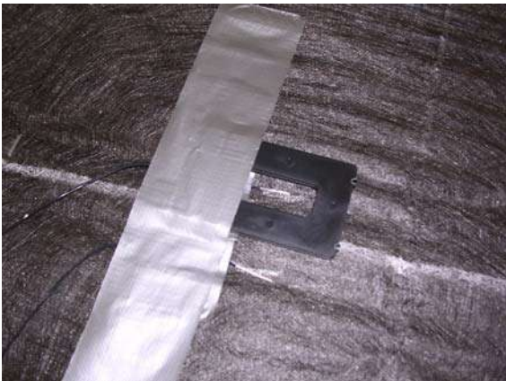
Figure 22: Sensor contact points with shim
