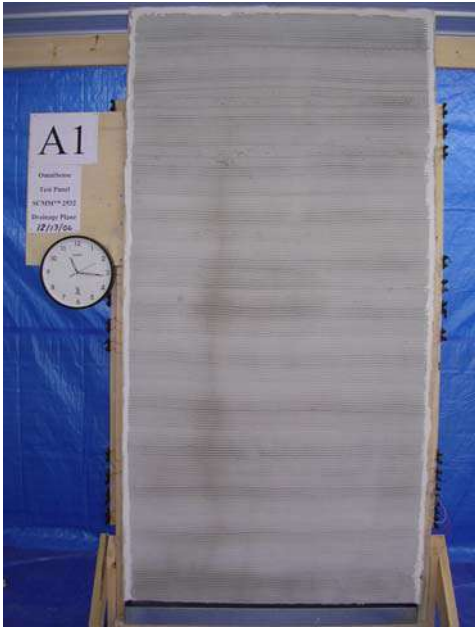
Figure 44: Panel A surface, 21 hours after spray application #1
