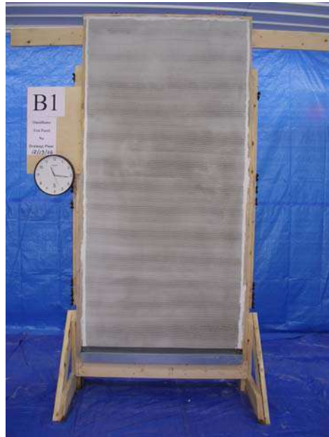
Figure 45: Panel B surface, 21 hours after spray application #1
