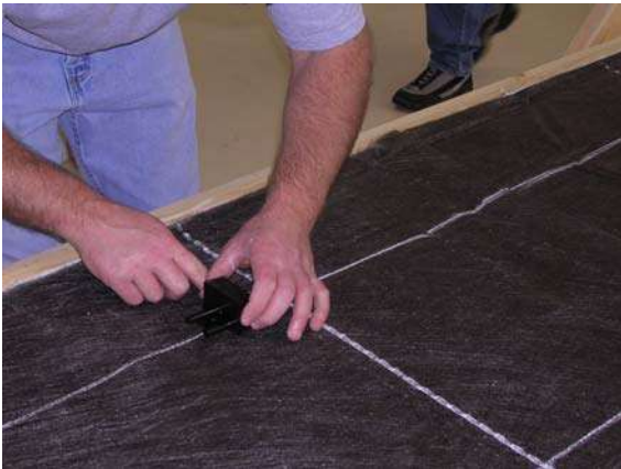
Figure 20: Marking sensor contact points
